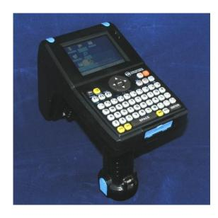
UHF HH RFID reader is the industry leading read range and read rate performance. It provides exceptional reading distance ie 6 M in open space and 10 M in indoor confined area. In addition, it gains the highest read rate ie 150 tags per second.
